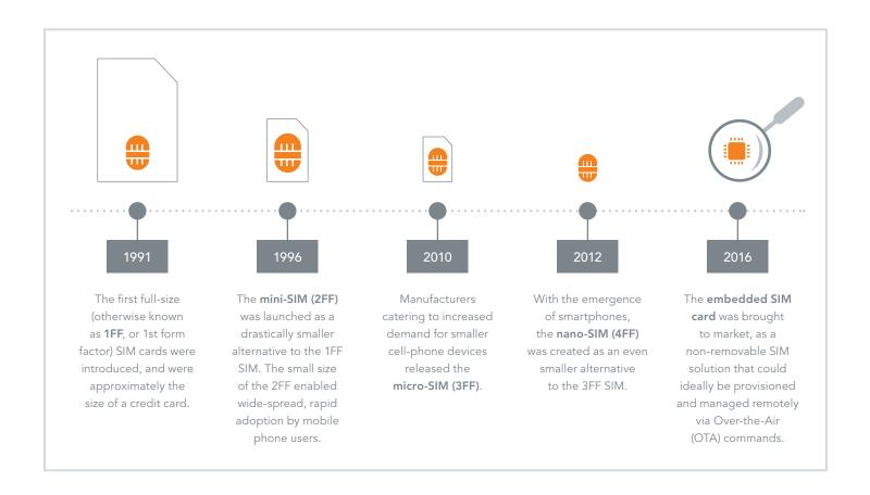
All SIM form factors are used in IoT, and the optimal selection is dependent on factors including the IoT device size, intended application, environment, etc.
